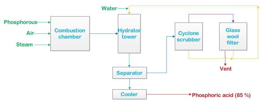
Figure: Manufacturing of Phosphoric acid by Oxidation and Hydration
